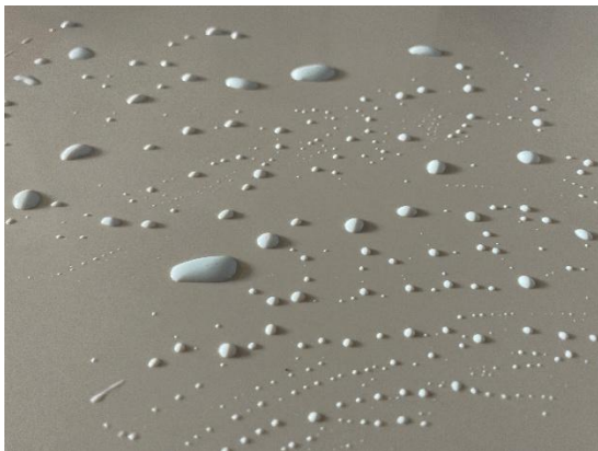
Tile with nano-treatment. The primer "retracts" and beads up.
